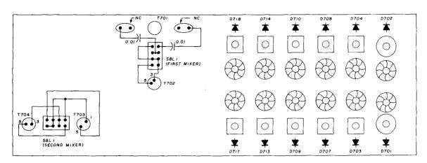
fig. 1. Circuit board *G* in the Heath SB-104A showing, at right, the locations of the original bandpass-filter switching diodes, which are replaced with MPN3401 PIN diodes to reduce loss through the circuit. The original first and second mixers on board *G* (center and left) are replaced with SBL-1 broadband mixers to reduce conversion loss and improve strong-signal-handling capability. Original Heath parts designators are shown.
